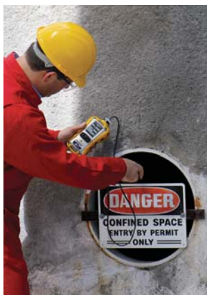
Confined space testing with the MultiRAE Lite
